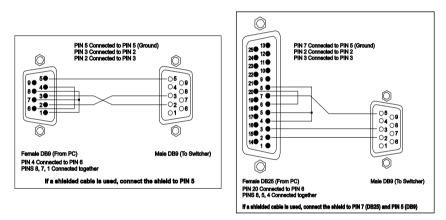
Figure 2: RS-232 Control Connector Wiring
