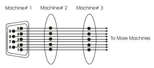
Figure 3: Connecting Multi-Machines
