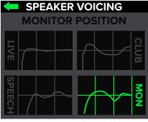
Simply rotate the speaker control knob until the speaker mode you desire is illuminated, then push to select it. As seen above, we selected Monitor.
