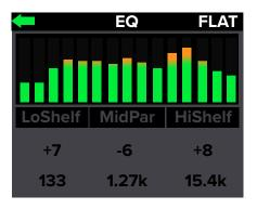
From here, rotate the speaker control knob until the parameter you want to change is illuminated. Push the speaker control knob in to select the parameter followed by rotating the speaker control knob clockwise (raise the gain / frequency) and counter-clockwise (lower the gain / frequency).
