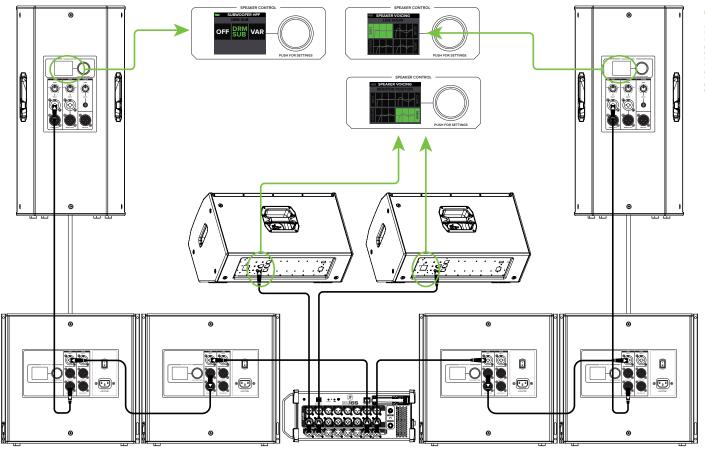
Here's how to set up a large club system. In this example, the L/R outputs of a DL16S mixer are connected directly to the CH1 inputs of a pair of DRM18S subwoofers. The Direct Out of each subwoofer is then connected to the inputs of an additional pair of DRM18S subwoofers. The X-Over of these subwoofers may be set to DRM Top.
