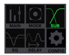
• Var – Choose this if a non-Mackie DRM18S subwoofer is connected to the system. Here you can select the subwoofer's HPF, ranging from 40 Hz – 160 Hz.
