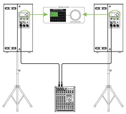
In this example, a ProFX8v2 mixer is connected directly to two DRM215 loudspeakers. It is the perfect setup for a small club or... a fun karaoke house party! Simply connect the L/R outputs of the ProFX8v2 mixer to the CH1 input of each DRM215 loudspeaker. Don't forget to set the Speaker Mode on both loudspeakers to Live... or Club if you want a little more low-end thump!
