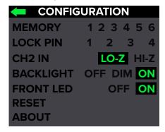
To change a setting, just rotate the speaker control knob until the configuration you desire to change is illuminated, then push to select it.
