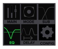
The DRM212, DRM215 and DRM315 all have 3-band EQ with shelving hi, peaking mid and shelving low. Shelving means that the circuitry boosts or cuts all frequencies past the specified frequency. Peaking means that certain frequencies form a "hill" around the center frequency.
