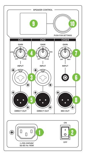
Also, channel 2 may accept a Hi-Z source (such as a guitar) via the 1/4" input without the need for a separate DI box. Be sure to set the Ch. 2 In to Hi-Z in the Configuration menu, though! Directions on page 17.
