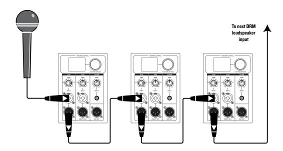
DRM loudspeakers may be daisy-chained via the male XLR connector labeled "DIRECT OUT" (which sends only the signal from the input located above it) or via the "MIX OUT" which outputs all inputs. Simply plug the signal source (i.e., mixer output or microphone) into the input jack(s), and patch that loudspeaker's direct out or mix out jack to the next loudspeaker's input jack, and so on, daisy-chaining multiple DRM loudspeakers. See above for visual representations of daisy-chaining.
