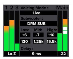
As you can see here, this is the same exact look as the default main screen. Like the default main screen, here you can only update the main output level. Do so by turning the speaker control knob clockwise (louder) and counter-clockwise (quieter). Once the level you desire has been dialed in, press the speaker control knob again to return to the main screen.
