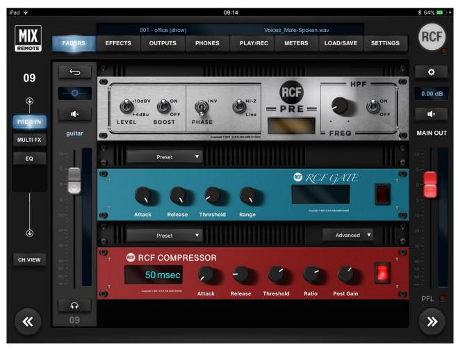
The -10dBV and +4dBu options are similar to the other line-level inputs; the **Boost** option allows you to insert another 2 dB boost to the analog stage; while the **Hi-Z** option enables a real high-impedance stage to get the best sound from your passive instrument. When in Hi-Z mode, the impedance is 1 M $\Omega$ . When using active instruments, we suggest maintaining the Hi-Z option OFF.
