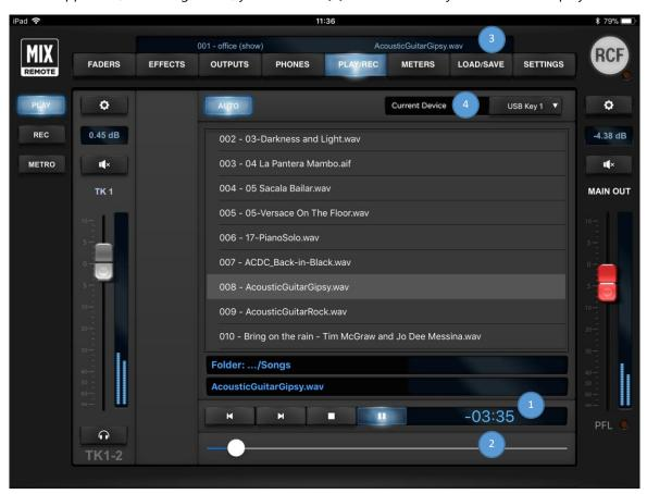
A large selection pane allows you to navigate through the USB flash drive folder (upper section), and then to select the specific files (lower section). To navigate to the previous directory, in the folder section, you can click on the line with 3 dots. *Please notice that with a very large amount of files, it takes several seconds to show all file names.*
