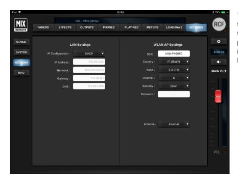
Two sections are accessible from the NETWORK view: on the left side, for the wired LAN port; on the right side, for the internal Wireless LAN Access Point.
