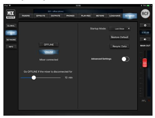
In case of communication issues between the tablet and the mixer itself, you can press **Resync Data**, which recalls the last active status of the mixer, including all the changes done.
