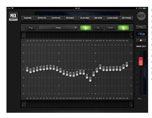
On the upper side there are: **Preset** dropdown to save and recall your custom settings, **DRAW** button that allow to manually design your equalizer curve, **2x** button to double the size of bands for a more accurate editing, **FLAT** button to set all bands to 0 dB and **ON** button to enable or disable the GEQ.
