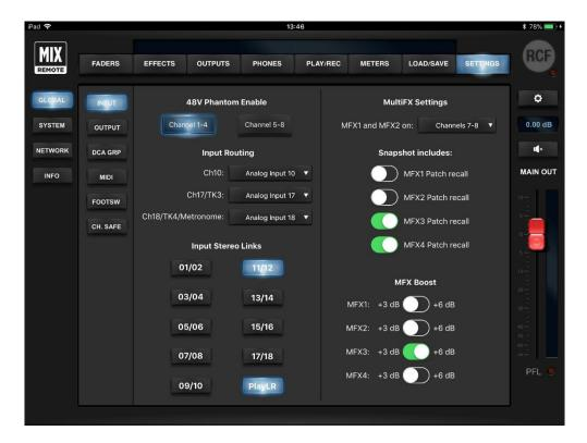
The **48V Phantom Enable** section allows the activation of 48V phantom power for microphone inputs in groups of four, using Channel 1-4 and Channel 5-8 buttons.
