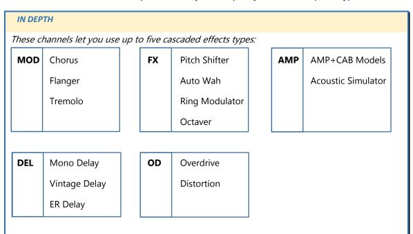
You can change the order of cascaded effects through the selector Order, and view the result on the top right indicators. These indicators show the ON/OFF status, an also allow you to select which pair of effect is visible on the central section for editing. The order from left to right of the FX, OD, AMP, MOD and DEL buttons reflect the actual audio cascading.
