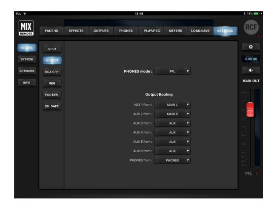
The **Phones Mode** section allows selecting between **PFL** (on FADERS INPUT page) and **Personal Mix** for the headphone output.
