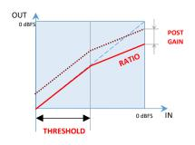
For faster adjustments, the compressor features the **Easy** option, located in a small box on the left of the Preset box - Easy has only the **COMPRESSION** control (based on input level signal with preset thresholds, with automatic Post Gain adjustment) against the five controls of **Advanced** option.
