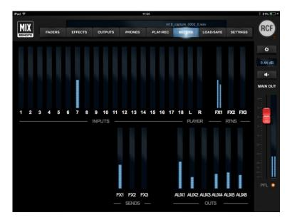
This tab has just page, which provides an instant view of the levels of all INPUTS - including the PLAYER – and of three FX stereo returns (RTNS).
