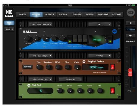
The left column shows the SEND and the MULTIFX select buttons; the right column shows usual the MAIN OUT controls.
