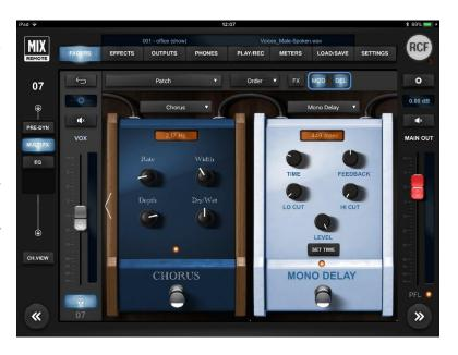
At the top of each pedal there's a display showing the last modified control value. At the bottom there's the activation switch; its status is displayed by a light which is lit when the unit is on.
