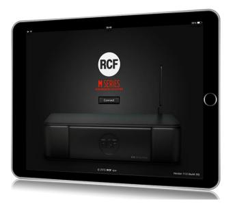
MixUpdate is a dedicated application for M 18 firmware update. MixUpdate for iOS also features BACKUP and RESTORE functions. BACKUP allows saving all the Snapshots, Shows and Effects' Patches from the mixer into a USB stick inserted in the M 18. Then, the RESTORE command brings the contents back to the M 18, either the same unit or a different one.
