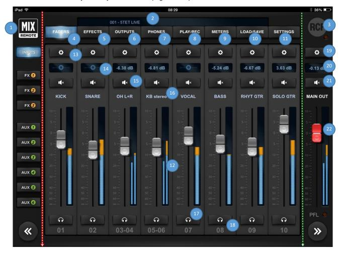
In the central area, on the upper side, there is a small text box with indications of the currently active session (2). Below there is a row of main tabs, named from left to right FADERS (4), EFFECTS (5), OUTPUTS (6), PHONES (7), PLAY/REC (8), METERS (9), LOAD/SAVE (10) and SETTINGS (11); the active tab is backlit. On the right side there's the RCF logo (3), which is lit (in brilliant white) when your controller is connected to the M 18 Digital
