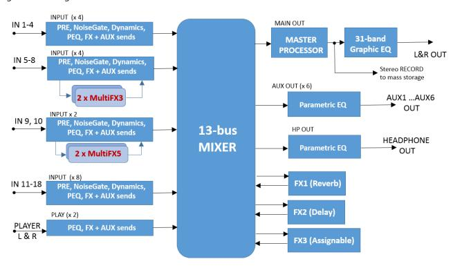
Signal processing capabilities of the M 18 Digital Mixer
