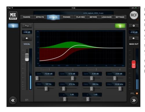
Pressing \*, you recall the OUTPUTS EQ page, containing the Advanced EQ for that AUX send; the other controls are for level and mute.
