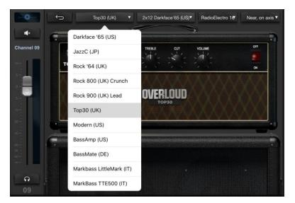
The ON/OFF rocker switch represents the BYPASS switch, and has same function as the switch on the stomp box view. As visible on the left, most Cabinets have similar names to the Head AMPs.
