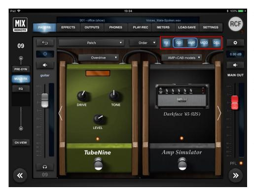
At the top of each pedal there is a display showing the last edited control value. At the bottom there is an activation switch; its status is displayed by a light, which is lit when the unit is on.
