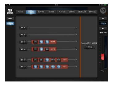
The four channels that have multiple effects are shown on the EFFECTS > MULTIFX page. Here you can also configure which pair of channels - Channels 05-06 or Channels 07-08, which are active in this example – will have the MFX option active. With the Settings button it's possible to jump directly to the SETTING > GLOBAL > INPUT page and change the MFX1 and MFX2 assignment. Only channels 09 and 10 provide you five effects.
