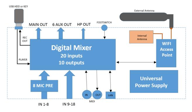
The internal Access Point is a dual-antenna MIMO WiFi interface; one of the two antennas is external, while the other is located on the top right side (when facing at the RCF logo).
