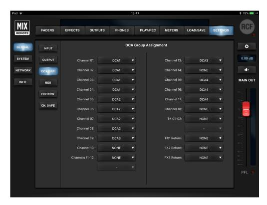
When a DCA Group is assigned to an input channel, the DCA group number is shown on top of the channel strip meter, so that you can easily visualize the assignment.
