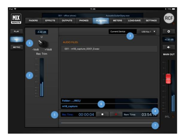
The file is auto-saved every ten seconds, so that any unwanted interruption (i.e., the USB storage device is removed abruptly, or M18 power is turned off) does not result in a total loss of audio data.
