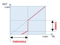
The second unit is the **RCF GATE**, topped by its **Preset** box, with **ATTACK** and **RELEASE** time controls, **THRESHOLD** level and **RANGE** intervention, completed by the display and the activation switch. On the left you can see the characteristic curve of the internal GATE: when the input signal goes below the THRESHOLD, its level is reduced by RANGE dBs.
