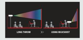
It can fit comfortably behind a presenter to eliminate long cable runs. As well as preventing shadows and providing a reduction in glare that may distract the presenter.
