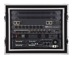
**TLM-170V:** 17" Full HD monitor which slides out from the topmost 1 RU slot. Features include Connections for SDI / HD-SDI and HDMI, Screen Markers (Center Marker, Aspect Marker and Safety Marker), Timecode Display Overlay, Scan Mode, Aspect Ratio Selection, Check Field, Waveform Overlay, Peaking Filter, Image Flip, HDMI/SDI Cross Conversion, False Color, and Embedded Audio Level Meter.
