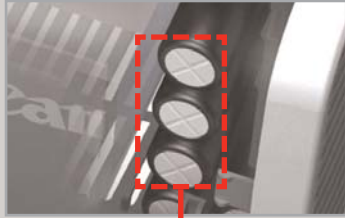
Internal charging system for cooling fan.
