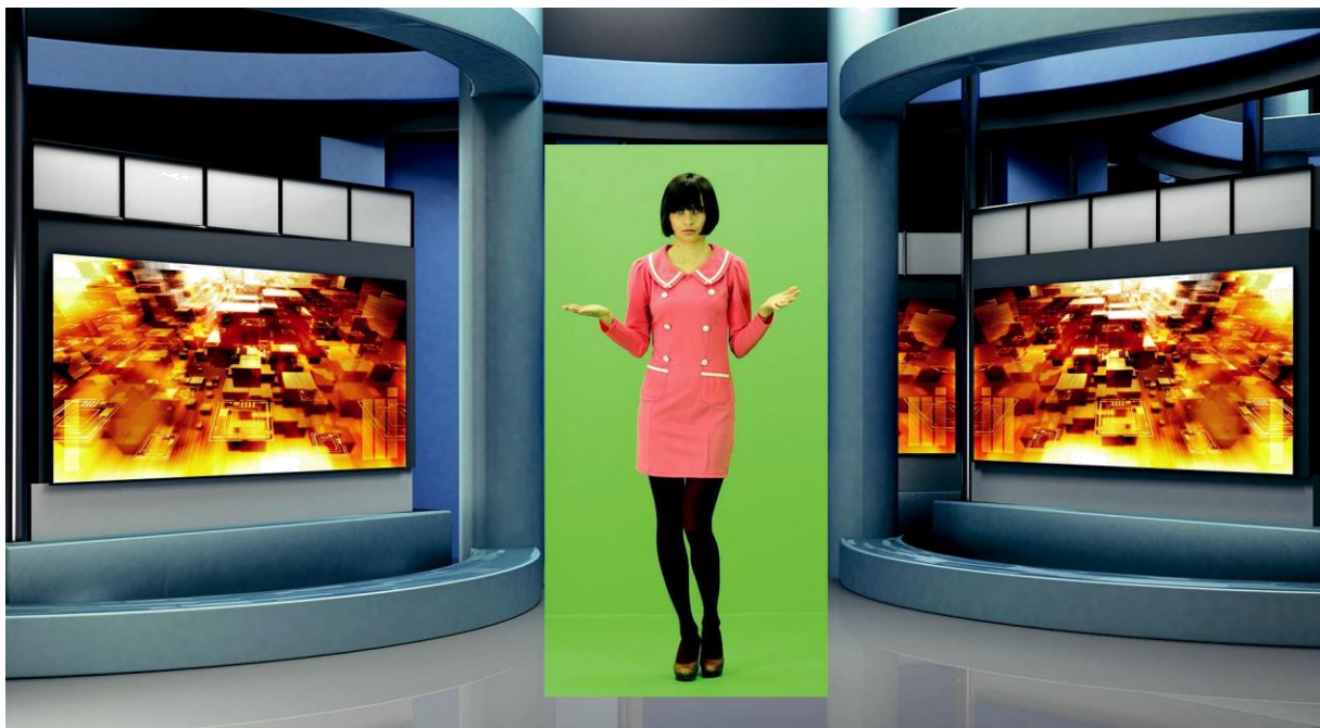
A view after a Garbage mask correction with the keying algorithm switched off
