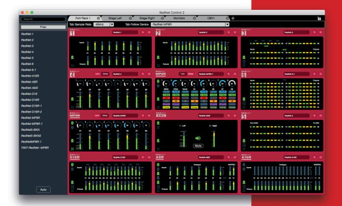
RedNet Control provides remote control and related functionality for the RedNet range of Dante-based audio-over-IP systems. The latest version, RedNet Control 2, has been completely revised, with a new tabbed browser-like graphic user interface and the ability to handle up to 600 RedNet devices and up to 96 channel of mic pre on one screen.
