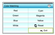
Red: Press the ▲ or ▼ to select Hue, Saturation and Gain Colors. Then press the ◀ or ▶ to decrease or increase the value respectively.
