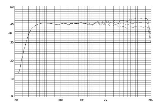
Figure 4. System 800A. Effect of HF contour on anechoic response.
