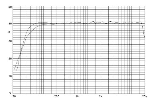
Figure 3. System 800A. Anechoic response. LF contour ON & OFF
