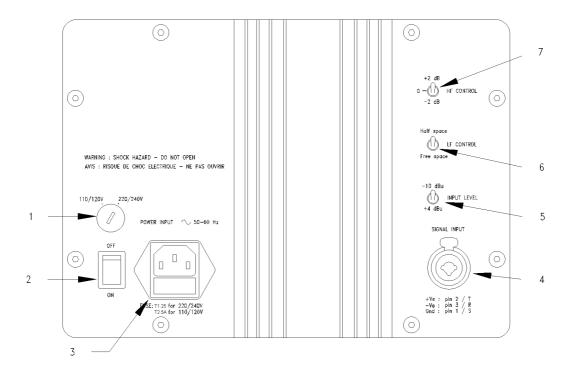
Figure 1. System 800A - Rear view
