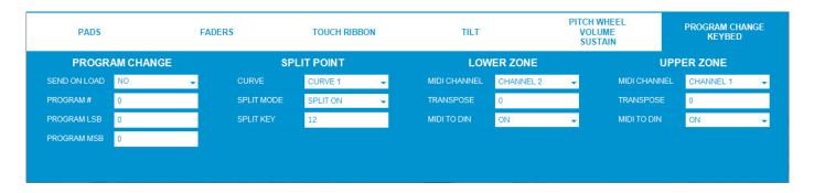
Click the **Program Change/Keybed** tab to set Program Change parameters for when presets are loaded and the MIDI assignments for Vortex Wireless 2's keys.
