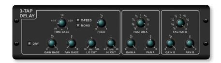
The **3-TAP DELAY** in the X32 PRODUCER records the input signal and then echoes it back after a user-definable period of time and number of repeats. What makes the stereo and triple delay useful and outstanding is the linked tap-timing and musical choice of echo patterns.
