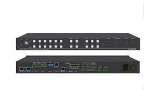
VS-622DT is an all-in-one 4K@60Hz (4:2:0) presentation system with 6x2 HDMI/HDBaseT matrix switching, control gateway, PoE, power amplifier, and Maestro room automation. The unit reclocks and equalizes the signals and can route any input to the HDMI or the HDBaseT output or to both outputs simultaneously. It supports resolutions up to 4K@60Hz (4:2:0) and WUXGA.
