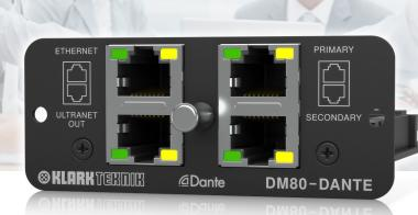
The DM80-DANTE is a multichannel audio interface expansion card that enables the KLARK TEKNIK DM8000 Digital Audio Processor to connect to external devices using the Dante high-performance digital media protocol to deliver audio over a standard Ethernet IP network. Dual RJ-45 connections share 16 x 16 channel networking of 24-bit / 48 kHz low-latency audio over Cat5e cable (max. 100 m / 330 ft.),
