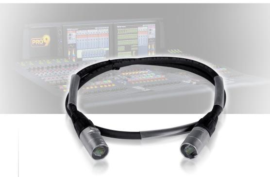
The CAT5E-1M ruggedised Cat5e bidirectional cable provides a digital audio network data link and features Neutrik etherCON NE8MC-1 connectors with an integral O-ring gasket to achieve IP54 water protection for high reliability, especially desirable in concert touring and festival applications. When used with MIDAS PRO and M Series and KLARK TEKNIK products equipped
