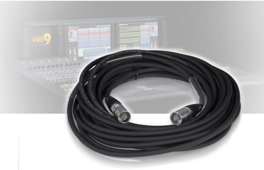
The CAT5E-10M ruggedised Cat5e cable provides a bidirectional digital audio network data link and features Neutrik etherCON NE8MC-1 connector carriers with an integral O-ring gasket to achieve IP54 water protection for high reliability, especially desirable in concert touring and festival applications. When used with MIDAS PRO and M Series and KLARK TEKNIK products equipped
