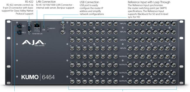
Fully Redundant AC Power Supplies Two independent 12VDC inputs provide safe operations. Power status can be checked from a LAN attached browser 3G-SDI Inputs and Outputs All inputs and outputs, 3G, HD-SDI, or SD-SDI (SMPTE-259/292/424)
