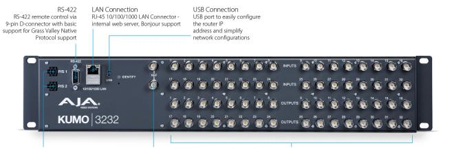
Fully Redundant AC Power Supplies Two independent 12VDC inputs provide safe operations. Power status can be checked from a LAN attached browser Reference Input with Loop Through The Reference Input synchronizes the router switching point per SMPTE specifications. The Reference Input supports Blackburst for SD and tri-level sync for HD 3G/HD/SD-SDI Inputs and Outputs All inputs and outputs, 3G/HD/SD-SDI (SMPTE-259/292/424/2081/2082)
