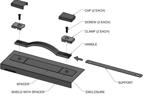
1. Remove the two screws from the right side of the enclosure and keep for reuse.
