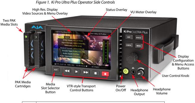
**Caution!** The AJA Ki Pro Ultra Plus contains a lithium battery soldered in place permanently (it is not user replaceable). If you ever dispose of the Ki Pro Ultra Plus, ensure you follow local regulations for safe disposal. The lithium battery shall not be exposed to excessive heat, such as sunlight or fire.
