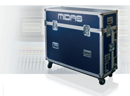
The PRO2-RC touring grade road case for the MIDAS PRO2 Live Digital Console is designed to withstand the rigours of live concert tours and is constructed from 12 mm thick rigid marine grade plywood with 40 x 40 mm durable aluminium edging extrusions. Composite density foam provides internal support and superior protection in transit, night after night, city after city.
