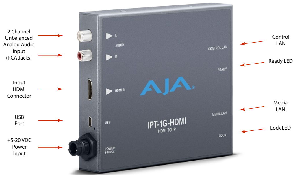
Figure 3. IPT-1G-HDMI Connections
