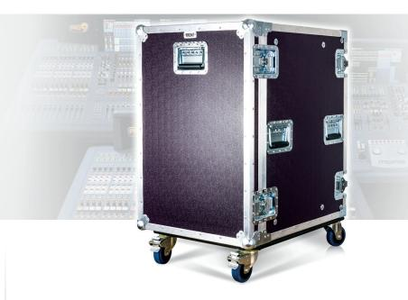
The PRO369-16U touring grade 19" rackmount road case for the MIDAS PRO3, PRO6, PRO9 and PRO X Live Digital Console systems is designed to withstand the rigours of live concert tours and is constructed from 12 mm thick rigid marine grade plywood with 40 x 40 mm durable aluminium edging extrusions. Designed to house both the MIDAS DL351 Audio System I/O stage
