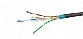
BCP-HDKat6 is a high-performance unified CAT6 Plenum rated cable that handles all Pro AV and IT signals over four overall screened twisted pairs This F/UTP CAT6 cable uses HDBaseT and Kramer's DGKat™ technology to pass video signals of up to 4K@60 (4:4:4) resolution. BCP-HDKat6 is also ideal for LAN applications.
