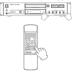
1. Press the **REPEAT/INTRO CHECK** [**PITCH**] button while pressing and holding the **DISPLAY** [**SHIFT**] button on the main unit or press the **PITCH** button on the remote control to turn pitch control ON. The current pitch control value is shown at this time.
