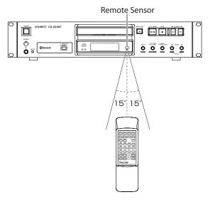
Operation distance Directly in front: Within 7 meters 15° left or right: Within 7 meters
