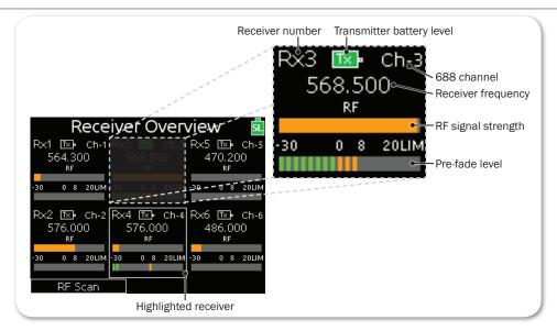
When supported by the transmitter, the transmitter battery level is indicated by the color of the battery icon: Green = over 50%, Yellow = over 20%, Orange = over 10%, Red = less than 10%. Whenever the transmitter battery level information is not supported by the transmitter, the icon is black.
