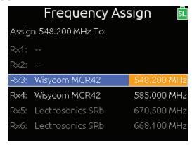
As shown in the illustration, the text of receiver channels that are available for assignment appear white. Gray text indicates receivers that are outside the range of the chosen frequency, and gray hyphens (--) appear when the SL-6 slot is empty.
