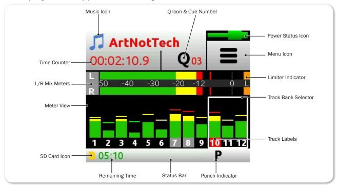
The sample image shows the Home screen on a MixPre-3, as indicated by the Track Bank Selector (white box) being around only three meters. This appears differently on the MixPre-6 and MixPre-10T.
