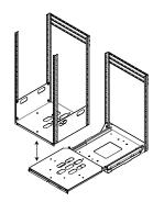
DOCKING: Rack can be removed from base for offsite integration.
