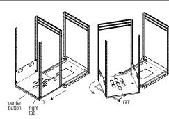
OPERATING: Slide Out: Grasp two front rails and pull rack firmly towards you, sliding it along rails in base. Rack locks in place when fully forward (0 degrees). Rotate: Press center button to release turntable and rotate rack left or right. Rack locks in place at 60 and 90 degrees. Slide In: With rack rotated back to 0 degrees, depress right tab to
