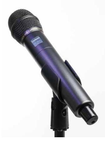
The transmitter benefits from a fourth generation design with specially developed, high efficiency digital circuitry for extended operating time on two AA batteries. The transmitter can tune across the UHF television band from 470.100 to 607.950 MHz, with a selectable output power of 25 or 50 mW. The pure digital architecture enables AES 256-CTR encryption for applications that require high level security.
