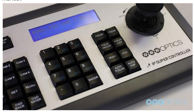
**Step 5** - The joystick is now ready to add cameras IP addresses. The SET UP button opens a menu on the LCD screen. Press the "ENTER" button to add a camera on setting "01/05" or "Add Camera". Set a Device ID for the corresponding camera o Input the camera's IP address into the joystick including the "." between octets. Example: IP = 192.168.100.88
