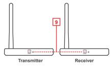
Channel selection can be done in 2 ways, manually press the button in front of the transmitter and the receiver or you can use the included remote to select the channels. To use the remote, simply point the included remote to the front of each unit after making sure that you have removed the plastic tab at the battery cover to enable the battery connection.
