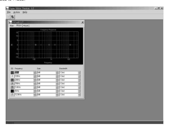
When you go to parameter equalizer, the PC will display above picture, you can adjust the frequency, gain, and bandwidth according to the application. If this unit is in LINK function, the change on channel A will be applied to channel B also. What's more, there are some small squares in the frequency contour, you can use these squares to adjust frequency, bandwidth and gain to achieve fast-start.
