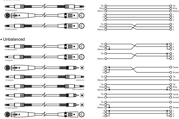
If you are connecting to a mixing console's main inserts, you may have a single TRS jack for Send and Return, in this case, use an insert "Y" cable that configured like the examples below.
