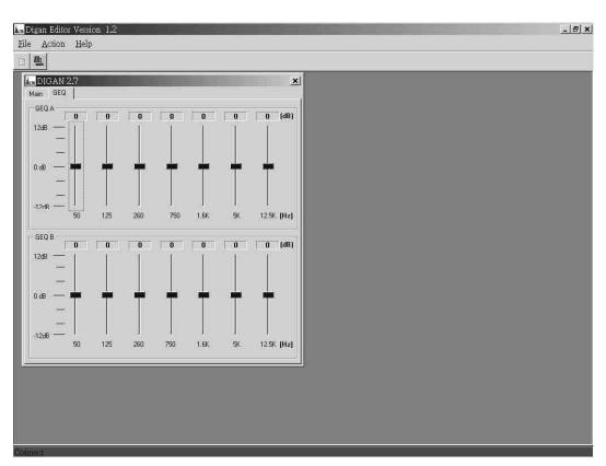
When you go to graphic equalizer, the PC will display above picture. You can adjust each band's gain value, if this unit is in LINK function, the change on channel A will be applied to channel B also. The adjustable range goes from 12dB to +12dB.
