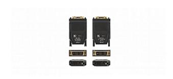
The 614T and 614R are a small and lightweight, detachable optical transmitter and receiver pair. They transmit uncompressed DVI resolutions of up to 1920x1200 at 60Hz using one multimode fiber optic cable with SC connectors. The 614T converts the DVI signal to an optical signal that it transmits to the 614R. The 614R decodes the optical signals back to a DVI signal.
