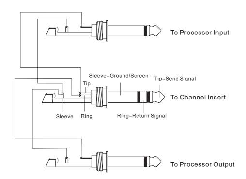
Y-Stereo lead for insert Connection
