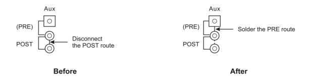
Modification on mono and stereo channels
