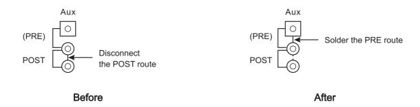
Modification on mono and stereo channels
