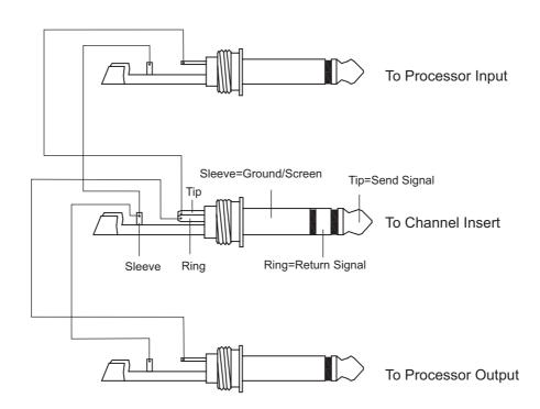
Y-Stereo lead for insert Connection
