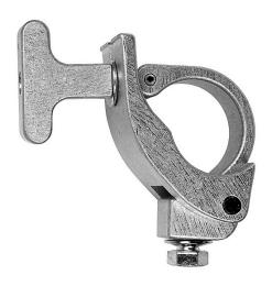
Lightweight profile for hanging small lighting fixtures to truss or pipes. Holds the weight of the fixture for you while you secure it. No set screw to ding truss. Fits from (I-I/4" pipe) I.66" OD to 2" OD truss tube. The Mini-Claw is a light duty clamp, and is not designed to side arm fixtures. The Mini-Claw has a I/2"-13 tpi by 3/4" long hex head grade 5 bolt for fastening to the fixture.
