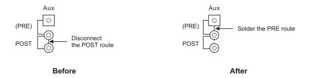
Modification on mono and stereo channels
