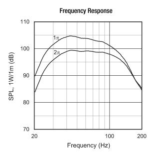
1 watt at 1 meter, with 150 Hz Linkwitz-Riley 4th order low-pass filter and 2nd order high-pass filter at 25 Hz with Q=2. 1pi (upper curve) and 2pi (lower curve) conditions.
