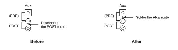
Modification on mono and stereo channels
