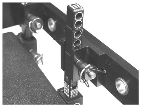
Figure 7: Alternate attachment using standard hingebar. Select hole zero (top VT4886 enclosure); attach at receiver block (hinge pin top radius – HPTR aligned at the bottom of the receiver block) so that hinge bar protrudes with 4 holes visible.
