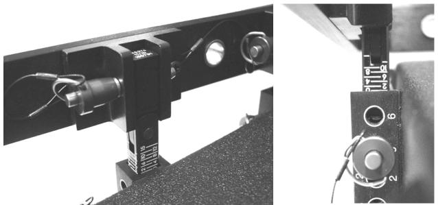
Figure 6: Select hole zero (top VT4886 enclosure) and the receiver block (hingebar recessed approx ½") to attach VT4886-SF to the VT4886 using the supplied adapter hinge bars.
