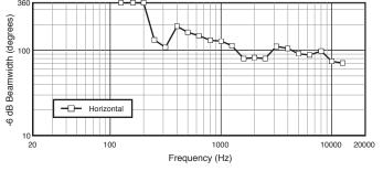
Horizontal Beamwidth, Single Element and Typical Array
