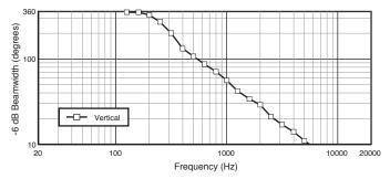
Vertical Beamwidth, Single Line Array Element
