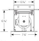
3/8" Threaded Rod (Not Included) Attached to Mounting Bracket
