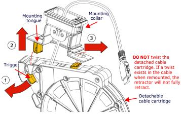
FIG. 4 HPX-AV102-HDMI-R MOUNTING COLLAR REMOVAL
