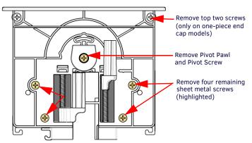
FIG. 2 HPX BASE ASSEMBLY - MOUNTING/PIVOT SCREW LOCATIONS
