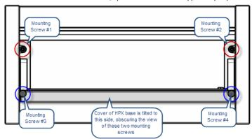
FIG. 8 HPX BASE ASSEMBLY (SHOWN MOUNTED) - MOUNTING SCREWS LOCATIONS
