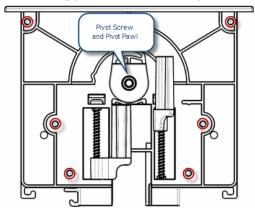
FIG. 5 HYDRAPORT BASE ASSEMBLY (SHOWN MOUNTED) - MOUNTING/PIVOT SCREW LOCATIONS
