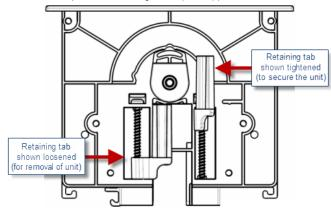
FIG. 4 HYDRAPORT BASE ASSEMBLY (SHOWN MOUNTED) - MOUNTING SCREWS LOCATIONS
