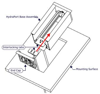
FIG. 6 INSTALLING THE HPX-N102-USB-PC MODULE
