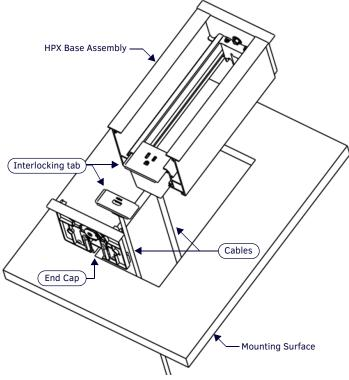
FIG. 2 INSTALLING THE HPX-P200-PC-US MODULE
