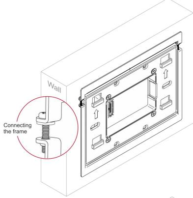
After hanging the KT-107 on the wall, tighten the two screws until the KT-107 is securely fixed in place.
