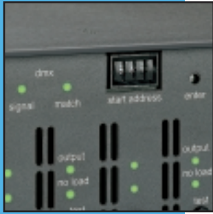
DMX SIGNAL AND DMX SIGNAL MATCH INDICATORS
