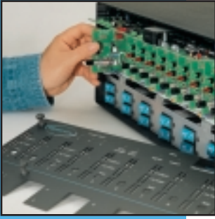
FRONT ACCESSIBLE POWER DEVICES
