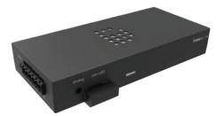
The DiGidot C4 Live is a small and powerful LED controller, that suits all kinds of situations. One device drives more than 6000 single LEDs. Furtermore, it supports 40+ addressable LED drivers and various industry standards. This is all you need in LED and showcontrol! With the built in user interface, the DiGidot C4 is easy to setup trough a web browser.
