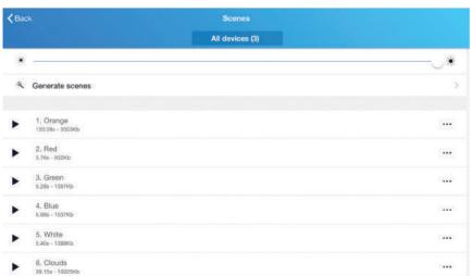
The DiGidot C4 Extended can record from Art-Net or DMX input and playback your scenes. This makes the DiGidot C4 Extended a stand-alone playback device in your setup.
