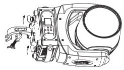
ALWAYS ATTACH A SAFETY CABLE TO THE FIXTURE WHENEVER INSTALLING IN A SUSPENDED ENVIRONMENT TO ENSURE THE FIXTURE WILL NOT DROP IF CLAMP FAILS.
