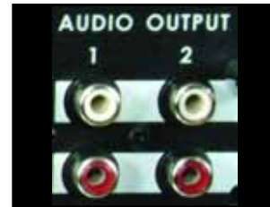
Audio Outputs 2 main and 1 earphone with volume control.
