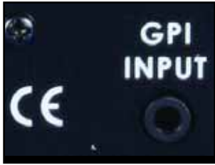
GPI Input Controls preprogrammed efx F01 to F30 in sequence.
