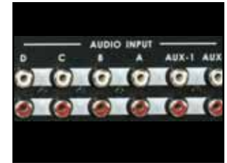
Audio Inputs 4 Stereo pairs and 2 Aux - Unbalanced audio.
